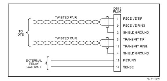
Figure D-3. DTE Drop/Insert (DSX-1) Cable
